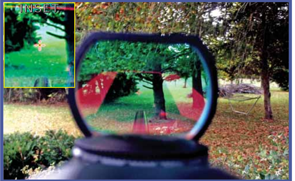
Left Photo: View through the Holo Sight from right of center. Note the position of the red dot in relation to the branches of the pine tree. Right Photo: This view is as it would be seen by a right hand shooter in a standard shooting position. Note that the red dot is still at the same point as in picture 4. See Inset, upper left corner, enlarged and enhanced so you can see red dot. (Author Photos)
