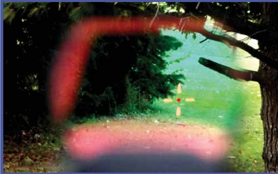
Left Photo: View through the Holo Sight from right of center. Note the position of the red dot in relation to the branches of the pine tree. Right Photo: This view is as it would be seen by a right hand shooter in a standard shooting position. Note that the red dot is still at the same point as in picture 4. See Inset, upper left corner, enlarged and enhanced so you can see red dot. (Author Photos)
