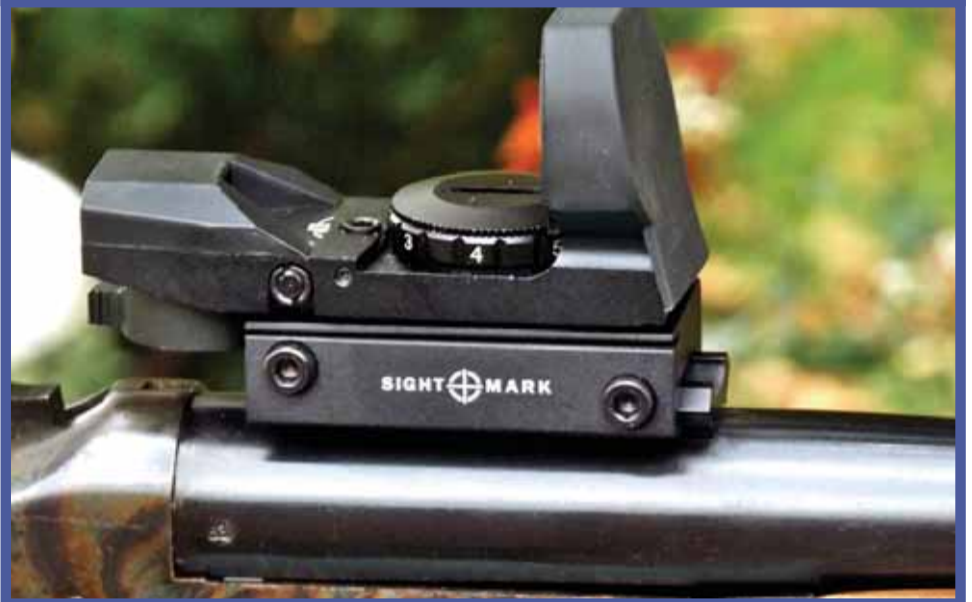
Top Photo: Springfield .410 single shot shotgun with Sight Mark Holo Sight installed on a Wilson Scope mount. Bottom Photo: Here is a Closeup view of the holo sight. You can see the shortened scope mount extending from the front of the sight. (Author Photos)
