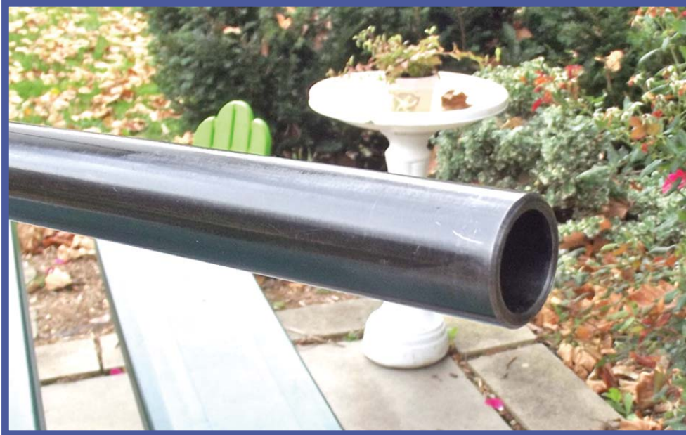
Close up of shortened barrel crown. The choke was opened up from full to an improved cylinder to better handle a rifled slug. (Author Photo)
