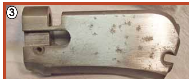
The old bluing and much of the rust has been removed. The extent of the pitting in the receiver is more evident. (Author Photo)
