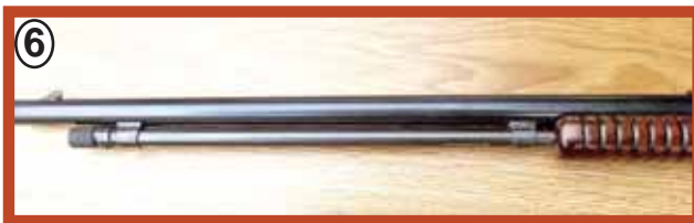
The magazine rings dove tails were repaired and the barrel finished. (Author Photo)
