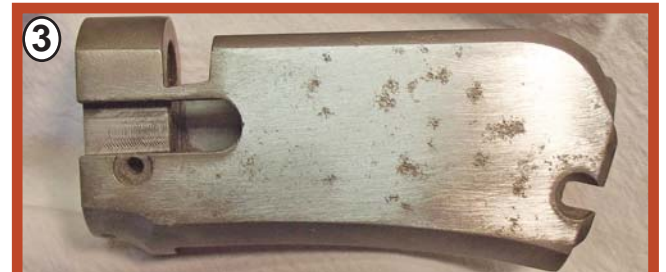
The old bluing and much of the rust has been removed. The extent of the pitting in the receiver is more evident. (Author Photo)
