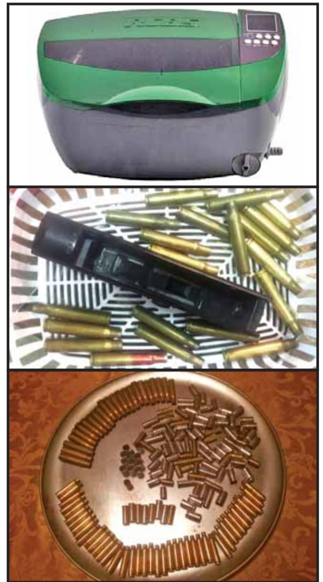
Top: RCBS Ultrasonic Cleaner. Middle: Carbon deposits left after first 30 minutes in cleaner. Bottom: Cleaned Brass had a bronze color after cleaning. (Author Photos)
