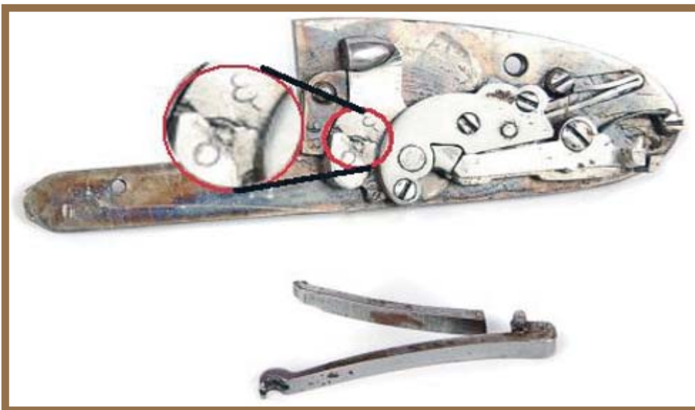
Look closely at the base of the hammer for the cracks in the metal. I've blown up the area in the inset and the cracks to make it easier to see. Picture is from B.K. Webster Gunsmith, Yorkshire England on the internet. (Author Photo)
