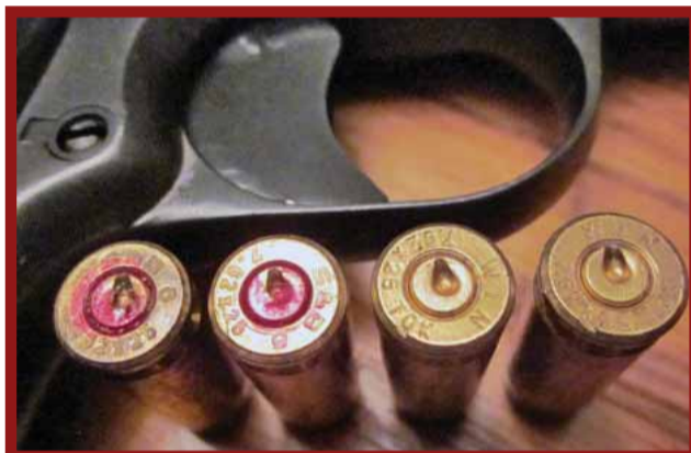
Firing pin wipe indicated here. Possibly due to early unlocking.
