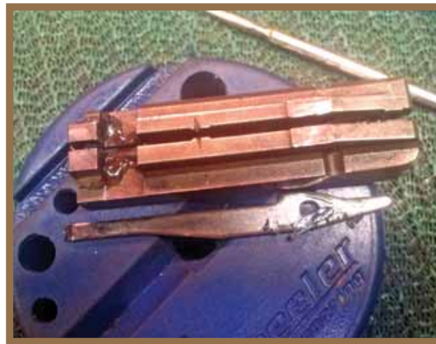
This is the bolt and firing pin. The pin was cemented inside the bolt and wouldn't budge. Heat was needed to loosen the firing pin for removal. (Author Photo)
