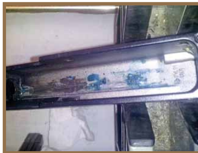
This is looking into the receiver with the bolt and trigger group removed. It's easy to see the 4 screws and where the blue Loctite® has hardened wedging the bolt and receiver together. (Author Photo)
