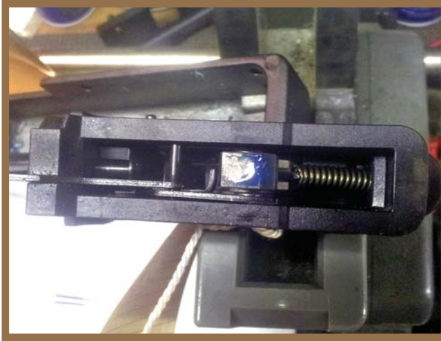
This picture is looking down into the trigger group. The blue loctite has migrated onto the top of the hammer. Luckily it had not gotten further into the trigger group. (Author Photo)
