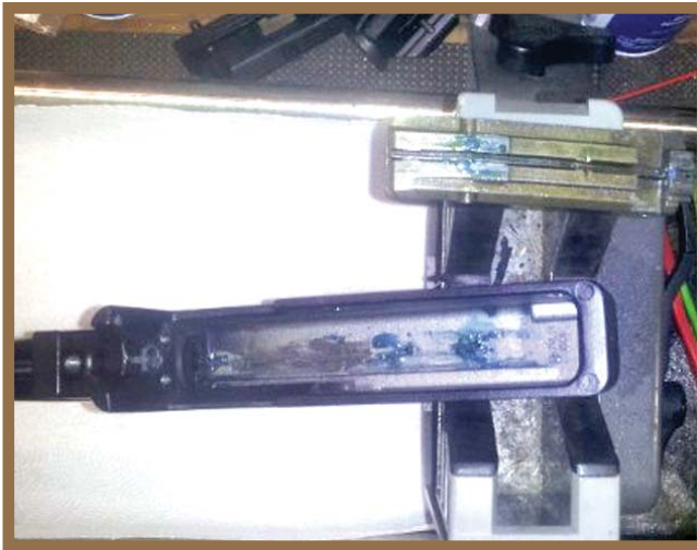
Here is a picture of the blue Loctite® inside the receiver and on the bolt. (Author Photo)
