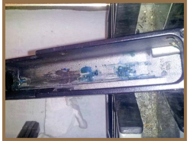
This is looking into the receiver with the bolt and trigger group removed. It's easy to see the 4 screws and where the blue Loctite® has hardened wedging the bolt and receiver together. (Author Photo)
