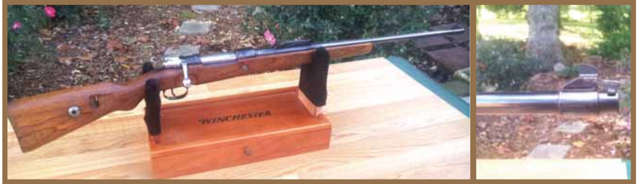
Left Photo: The rifle has been stripped of its bluing and polished to a low gloss. The original stock was modified to a sporting style stock with the bayonet hardware removed and the front sight "ears" removed. Right Photo: This photo of both sight blades shows the new installed sight next to the old sight. Note the .356" difference in the height of the blades. (Author Photos)
