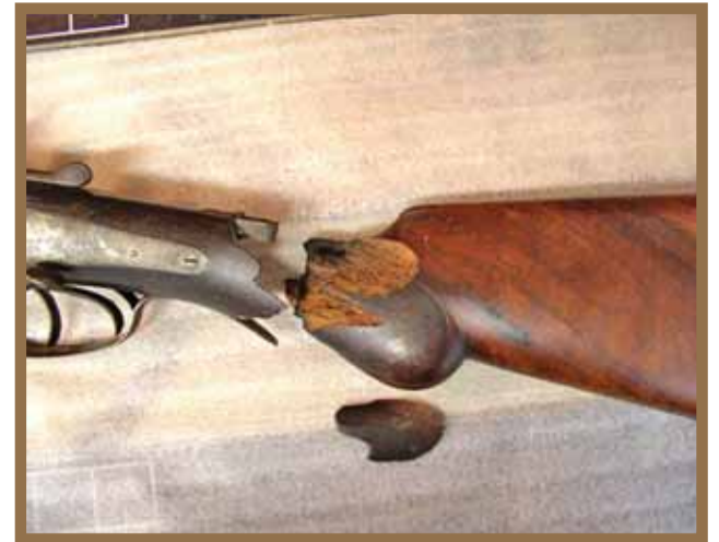
Right and left view of a broken stock. (Author Photo)
