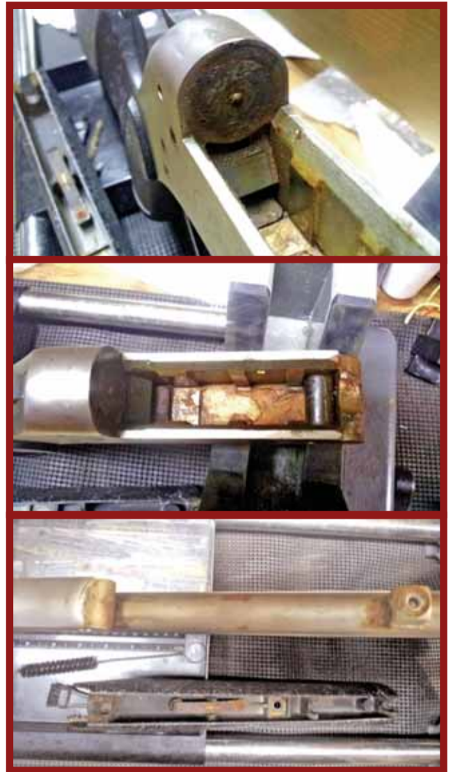
Top Photo: Here you see the breech face with the firing pin extended. The pin is not jammed by the corrosion but is on its way. This isn't rust but powder residue that will eventually pit and damage the breech face and firing pin. Middle Photo: This shows the inside of the receiver and the rust left by the moisture at the bottom of the receiver. Bottom Photo: Rust on the welded barrel lug will eventually cause it to fail. Note the rust on the barrel spring in the forearm below the barrel.. (Author Photos)
