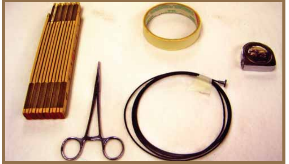
Tools of the trade. Carpenters folding rule, Wire cable to determine length of beam & tine, Masking tape to hold it in place, Forceps to mark the end & 1/4" tape to measure cable. (Author Photo)
