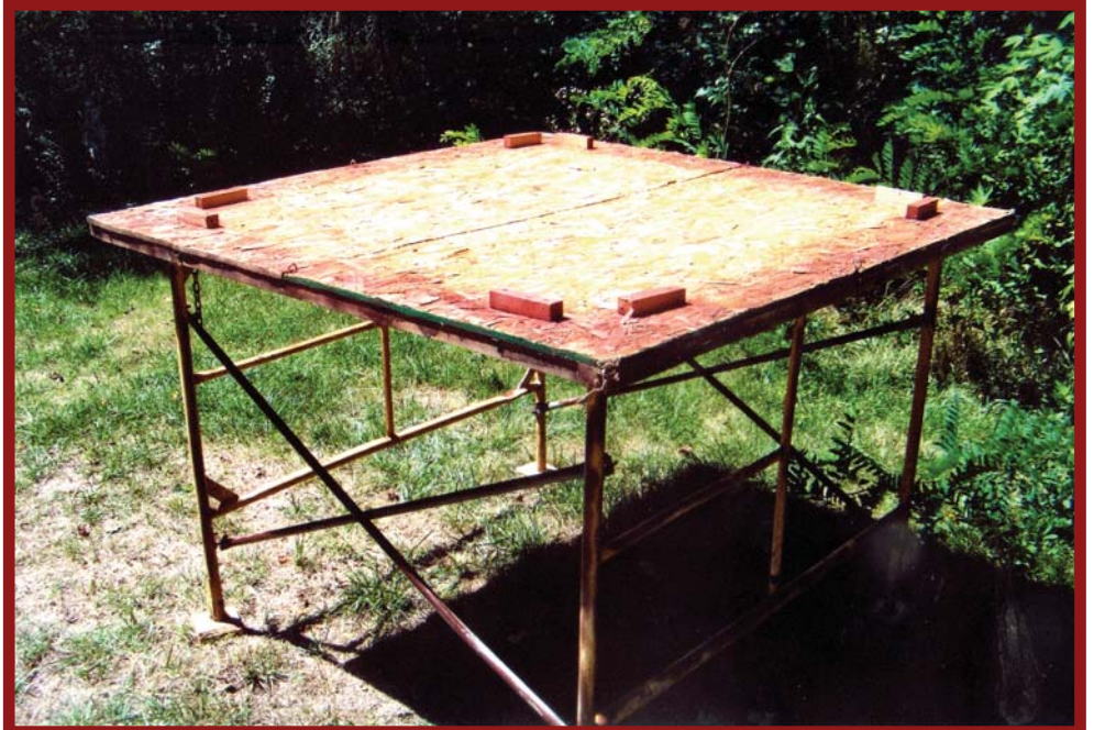
Picture #2: The floor, 1/2 inch particle board - 2 pieces - with corner blocks and eye screws in place. 2"x 2" material provides the frame and reinforcing. (Author Photo)
