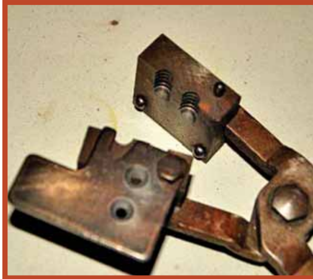
4. This is one type of bullet mold made of steel and made by RCBS. (Author Photo)
