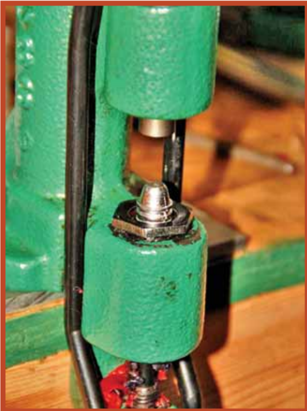
8. This is how the bullet is placed in the machine. The handle is pulled and the bullet is pressed down into a die forming it to the proper diameter and injecting the lube.
