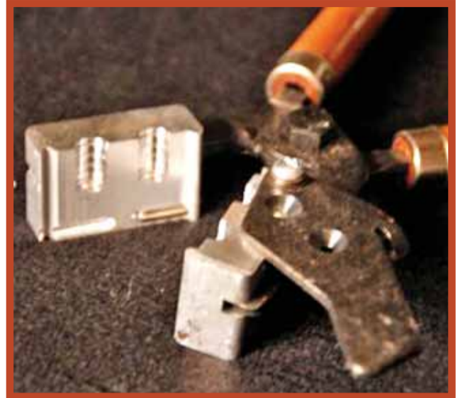
5. Here is a mold made of aluminum and made by LEE. They are cheaper but heat up pretty fast. You can get around this problem by using two of them, one cooling, one molding. (Author Photo)
