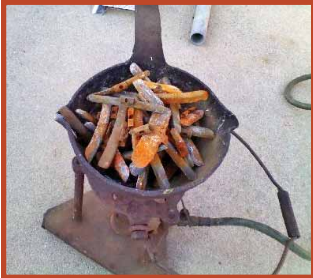
1. I start with used wheel weights. They're in an old ladle I picked up a number of years ago. (Author Photo)
