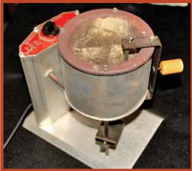
3. This is one of the melting pots I pour the metal into the bullet molds with. It is a bottom pour type. (Author Photo)
