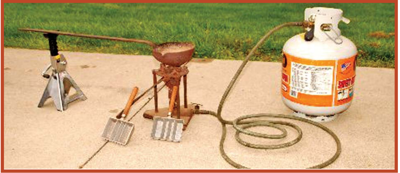
2. This is an old base for a plumbers pot used in the days when soil pipe was used for drains and required oakum and solder to seal it. Leaning against the base are a couple of molds to make 'pigs' which are then melted in the pot shown in the next picture. (Author Photo)
