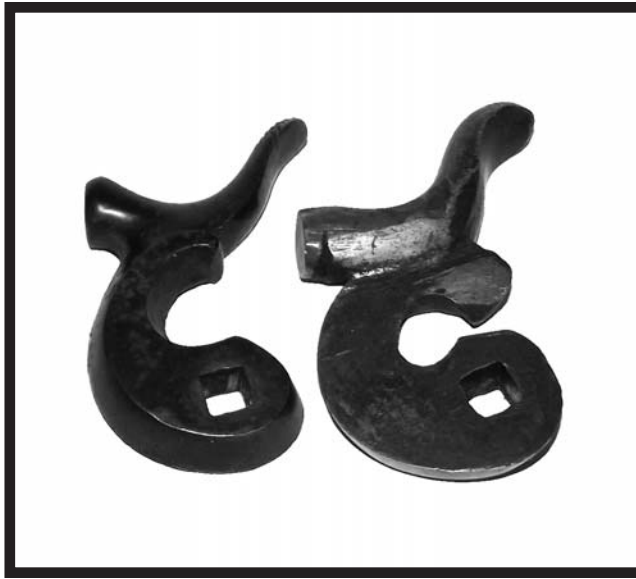
Left Photo: The Hammer Tumbler on the left has the screw still lodged in the piece. It appears to be a #4 or 5 size screw. If I can get it out without damaging the threads I'll be really happy. That part doesn't appear to be available. Right Photo: This picture was to show the differences in the two hammers. Both are for the L.C. Smith double. But are from different period of manufacture. (Author Photos)
