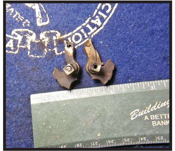
Left Photo: The Hammer Tumbler on the left has the screw still lodged in the piece. It appears to be a #4 or 5 size screw. If I can get it out without damaging the threads I'll be really happy. That part doesn't appear to be available. Right Photo: This picture was to show the differences in the two hammers. Both are for the L.C. Smith double. But are from different period of manufacture. (Author Photos)
